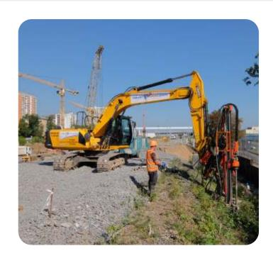
Drilling unit attachment Figaro can be easily mounted on existing equipment which provides required hydraulic system parameters.
